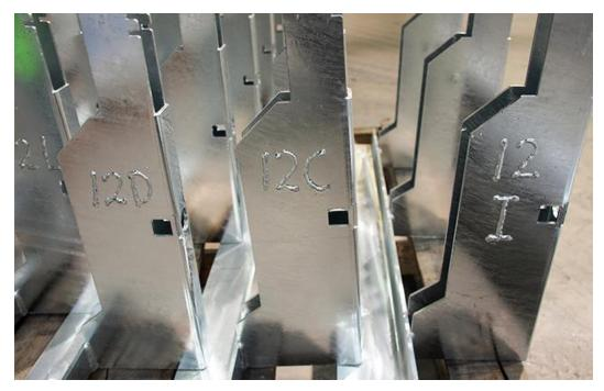
Fig. 3.2.5 Identity marks on material
