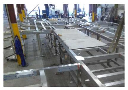
Fig. 4.2.1 Preparation of fabrication bed/platform in construction
