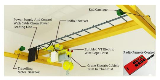
Fig. 4.2.3 Overhead lifting equipment (hoist)
