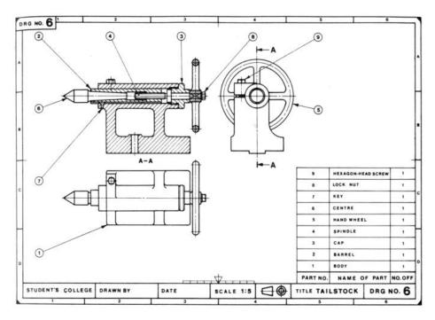
Fig. 3.1.5 Assembly diagrams
