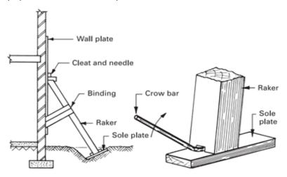
Fig. 5.1.4 Shoring installation
