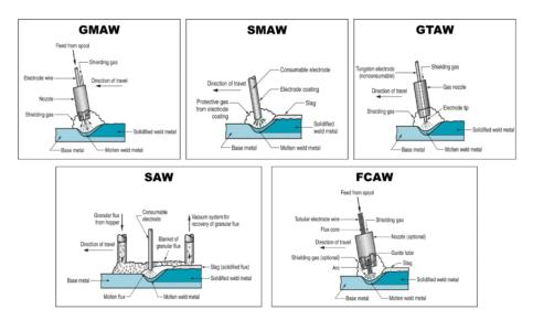
Fig. 4.1.20 Welding methods
