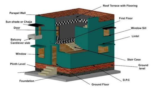
Fig. 3.1.15 Component identification
