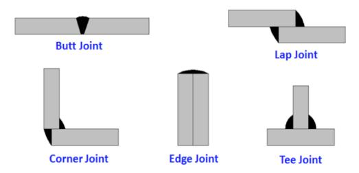
Fig. 4.1.17 Preparation of edges and joints
