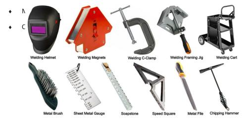
Fig. 4.3.16 Tools and equipment necessary for repair
