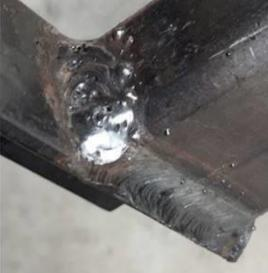
Fig. 4.3.5 Welding defects
