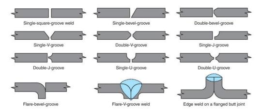
Fig. 4.1.18 Welding joint type
