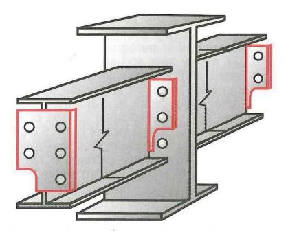
Fig. 4.3.13 Alignment correction for misalignment
