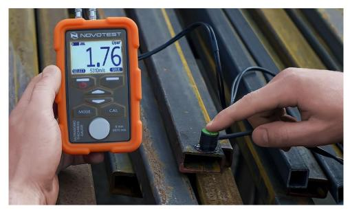
Fig. 4.1.21 Non-destructive testing (NDT)
