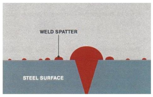
Fig. 4.3.11 Surface imperfections due to weld spatter
