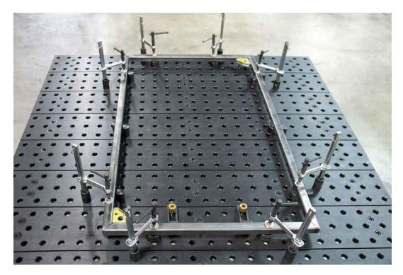
Fig. 4.3.4 Alignment and fixturing
