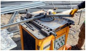
Fig. 1.1.11 Bar bending
