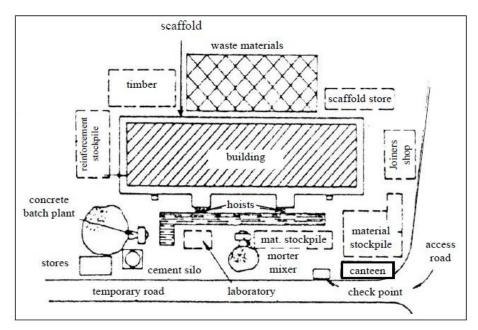
Fig. 1.1.18 Layout of a construction site
