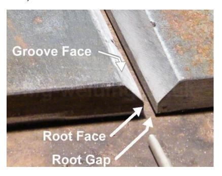
Fig. 4.3.1 Root gaps in joint preparation
