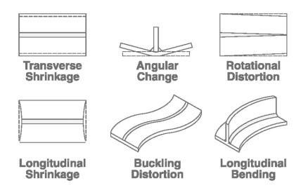
Fig. 4.3.3 Material shrinkage in welding
