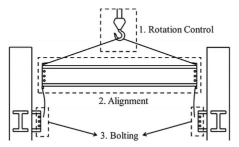
Fig. 5.3.2 Erection plan for aligning components
