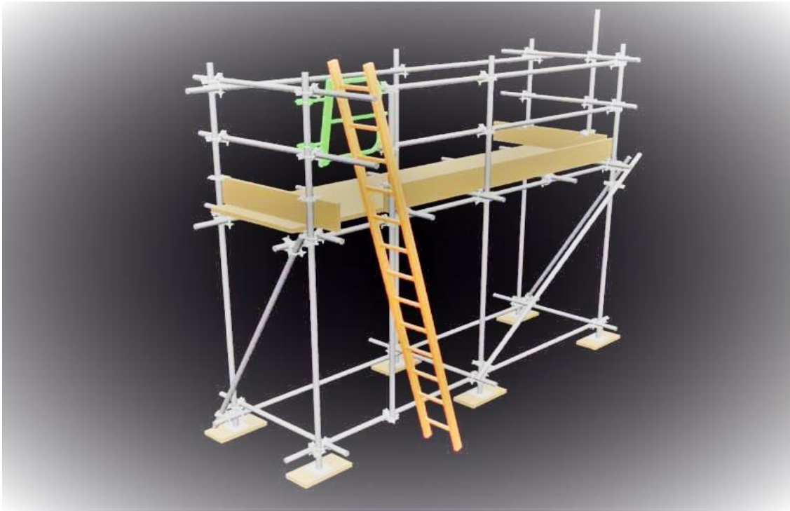
Fig.: 1 -Carryout double layer scaffold using pipe and coupler as per the following drawing.
